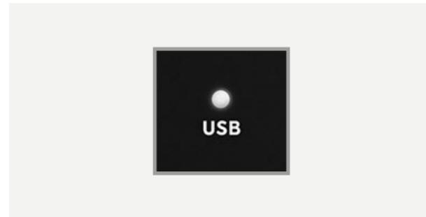
The white USB LED indicates connection via USB to your device. A solidly lit light means that there is stable communication between iD4 and the device.
