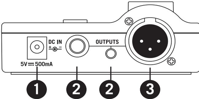
1. **DC Input** - Connect the supplied adapter here. **WARNING:** Do not substitute any other kind of power adapter. Doing so can cause severe damage to your RXD1m and void your warranty.
