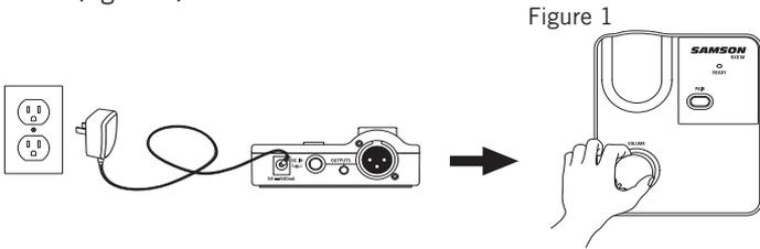
3. With your amplifier or mixer powered off and volume control down connect the RXD1m receiver output jack to the mic or line input using the balanced XLR output, unbalanced 1/4" or 1/8" output jacks. Turn the RXD1m power on but keep the volume at minimum level (figure 2).
