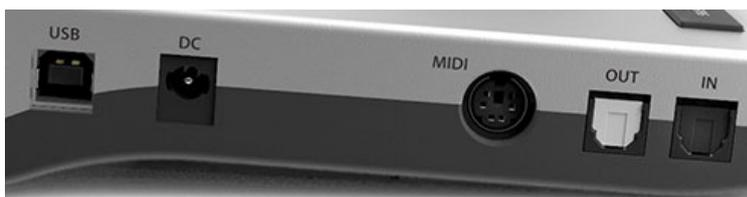
The left side of the Babyface Pro has an optical input and output, a power supply connector, a USB socket and a 6-pin MINI DIN connector for the included MIDI breakout cable.
