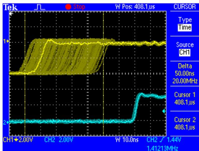
The screenshot shows an extremely jittery SPDIF signal of about 50 ns jitter (top graph, yellow). SteadyClock turns this signal into a clock with less than 2 ns jitter (lower graph, blue). The signal processed by SteadyClock is of course not only used internally, but also used to clock the digital output. Therefore the refreshed and jitter-cleaned signal can be used as reference clock without hesitation.
