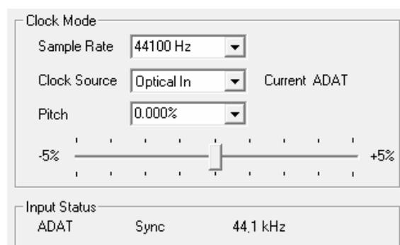
This way, configuring any suitable audio application for digital recording is simple. After connection the Babyface Pro displays the current and external sample frequency. This parameter can then be changed in the application's audio attributes (or similar) dialog.
