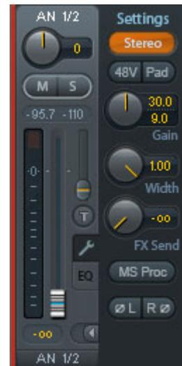
Input channels 3 and 4 are found as TS jacks on the right side of the Babyface Pro. These Hi-Z **universal inputs** have an input impedance of 470 kOhm. The input gain is controlled and performed digitally and limited to 9 dB. An additional hardware-based reference level optimizes the signal to noise ratio. Choices are +4 dBu and -10 dBV.
