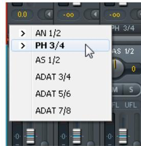
An arrow is only shown with an activated routing. A routing is seen as activated when audio data is sent. As long as the fader is set to  $-\infty$  the current routing will be shown in bold letters, but not have an arrow in the front.
