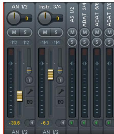
The **arrow symbol** at the bottom minimizes the channel width to that of the level meters. Another click maximizes it again. A mouse click with held Ctrl key causes all channels to the right to enlarge and minimize at once.
