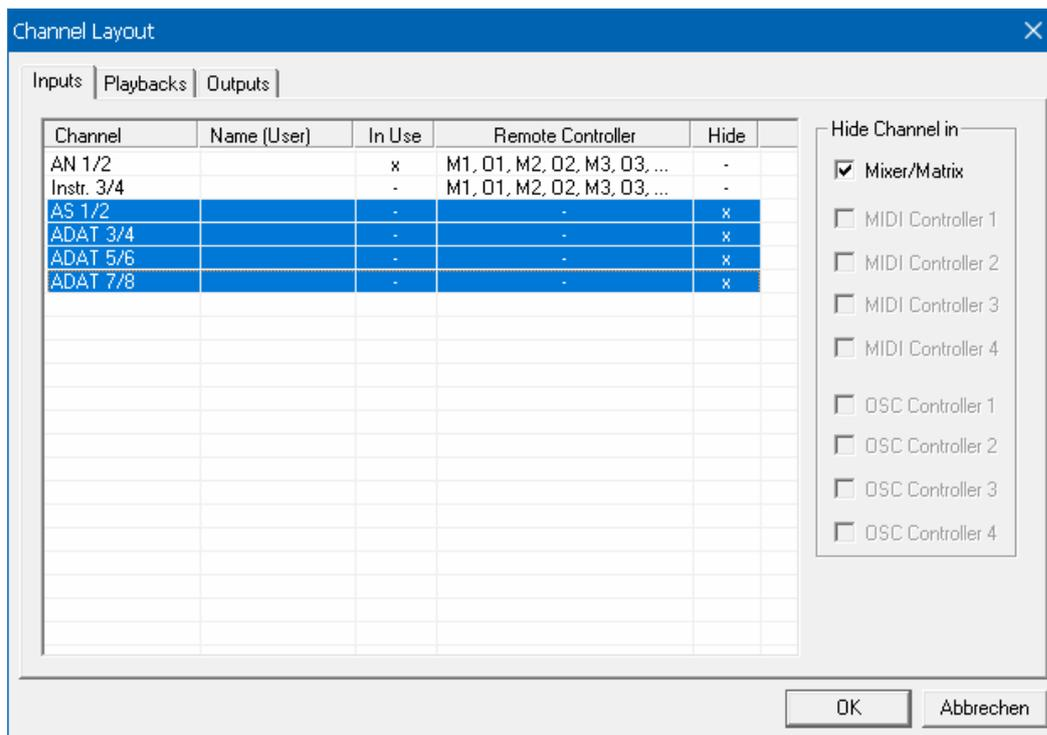
The dialog can be called directly from TotalMix by a right mouse click on any channel. The corresponding channel will then be preselected in the dialog.
