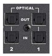
Running in S/PDIF mode, the optical i/o provides the option to integrate external digital outboard, allowing upto 4 channels of audio in and out of the iD44 at sample rates up to 96KHz.
