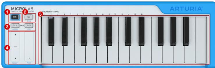
1. **Shift button:** This button lets you access the secondary functions of MicroLab. The secondary functions are listed in blue text under the buttons and strips and in black above the first 16 keys of the keyboard. These functions are described in the "Shift Functions" section later in this chapter.
