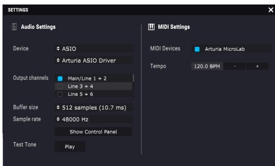
If MicroLab (or any MIDI controller) is connected to your computer, the Audio MIDI Settings window will reveal a section labeled "MIDI Devices". In this section, check the box labeled "Arturia MicroLab" so that you can use it to play Analog Lab Lite.
