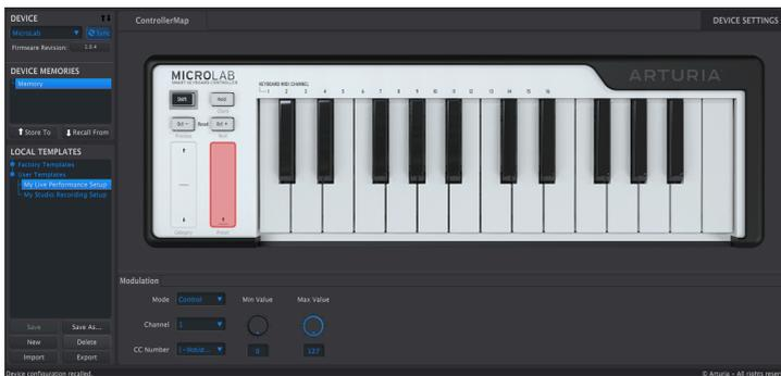
Editing MicroLab parameters in MCC is simple. A visual representation of MicroLab is shown on the right and various editable parameters are shown in the area below the image. Device Memories and Local Templates are displayed in the left column, but these features are not really necessary when using MicroLab due to MicroLab's minimalist feature set. As a result they are not covered in this guide.
