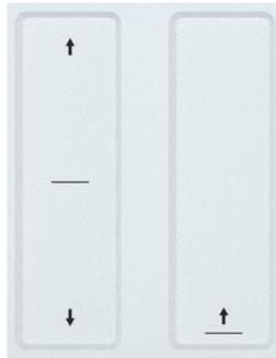
The touch-sensitive pitch and modulation strips are low-profile controllers that offer a different take on the traditional “wheel” design while maintaining their expressiveness. If you touch the Pitch bend strip at its center and move your finger forward or backward it will raise or lower the pitch of the played sound. Similarly, moving your finger along the Modulation strip alters the modulation amount of the played sound, from no modulation (bottom) to maximum modulation (top).
