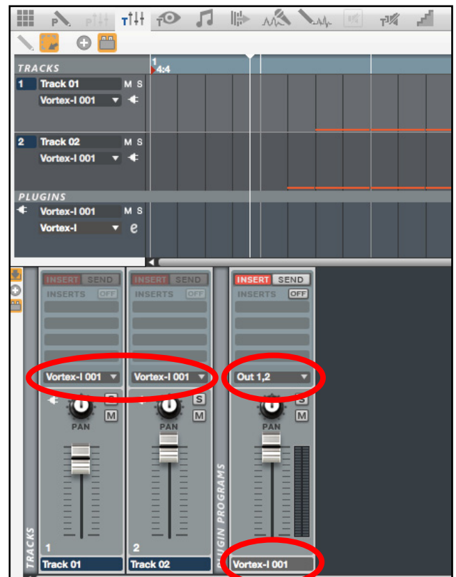
Track Mixer Mode. Tracks 01 and 02 are routed to the Vortex-I 001 Plugin Program, which is then routed to Out 1,2 .
