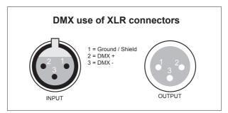
A word on termination: DMX is a resilient communication protocol, however errors still occasionally occur. Termination reduces signal errors, and therefore best practices include use of a terminator in all circumstances. If you are experiencing problems with erratic fixture behaviour, especially over long signal cable runs, a terminator may help improve performance.
