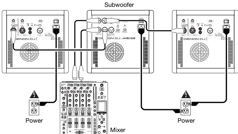
Using XLR or 1/4" (6.35 mm) TRS cables, connect the left and right output of your mixer to the inputs of your subwoofer, and then connect each high-pass output of the subwoofer to **Input 1** of each loudspeaker. Make sure the **Line/Mic Selectors** are set to **Line**.
