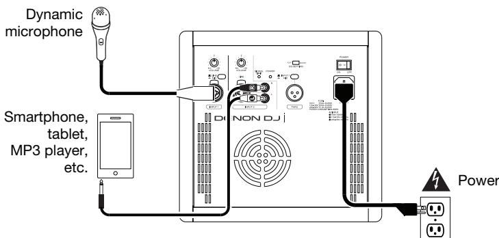
Connect a dynamic microphone to **Input 1** using an XLR or 1/4" (6.35 mm) TRS cable. Make sure the **Line/Mic Selector** is set to **Mic**. Connect a media player (smartphone, tablet, MP3 player, etc.) to **Input 2**'s RCA connectors using a 1/8"-to-RCA (3.5mm-to-RCA) cable.
