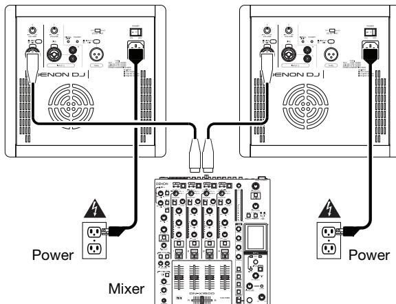
Connect the left and right output of your mixer to **Input 1** of each loudspeaker using XLR or 1/4" (6.35 mm) TRS cables. Make sure the **Line/Mic Selectors** are set to **Line**.
