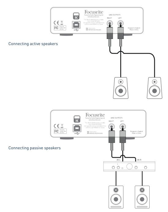
The line output connectors are standard phono (RCA) sockets. Typical consumer (hi-fi) amplifiers and small powered monitors will have inputs on phono (RCA) sockets or a single 3.5 mm 3-pole jack plug (intended for direct connection to a computer). In either case, use a suitable connecting cable with phono plugs (RCA jacks) at one end.
