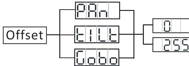
To enter the offset adjustment submenu, press the ENTER button for at least 5 seconds. In this submenu you are able to adjust the pan and tilt home positions and gobo wheel home position.
