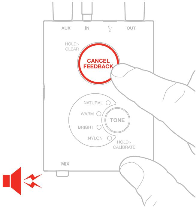
In case of a feedback tap the “CANCEL FEEDBACK” button and the troublesome frequency is instantly notched out of the mix, thus eliminating feedback without sacrificing tone quality. This feature set individuals notch filters (up to 10) for multiple feedback frequencies.
