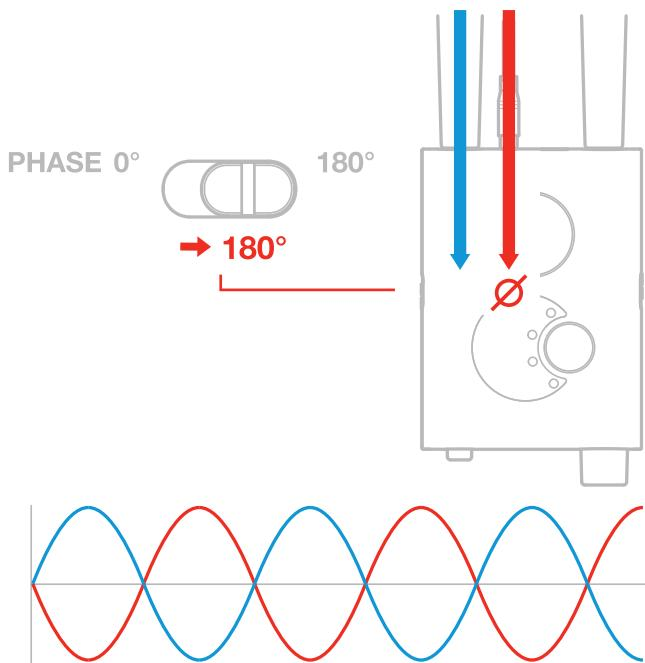
The phase flip switch ( $0^\circ$ - $180^\circ$ ) works pre-mix. When both the MEMS and the Piezo are connected the phase switch acts on the MEMS signal. When only the MEMS is connected it act on the MEMS signal. When only the Piezo is connected it act on the Piezo signal.
