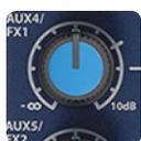
Signature 22 and 22MTX consoles have two internal FX processors and therefore have an additional Aux/FX send (Aux5/FX). The Aux 4 bus and the FX bus (also Aux 5 / FX 2 busses for signature 22 / 22MTK) are independent, but share the same Send level. The source for an FX bus send is always post-fader so that a source's contribution to an effect is proportional to its contribution to the mix. The Aux source can be switched Pre or post (as per normal Aux send).
