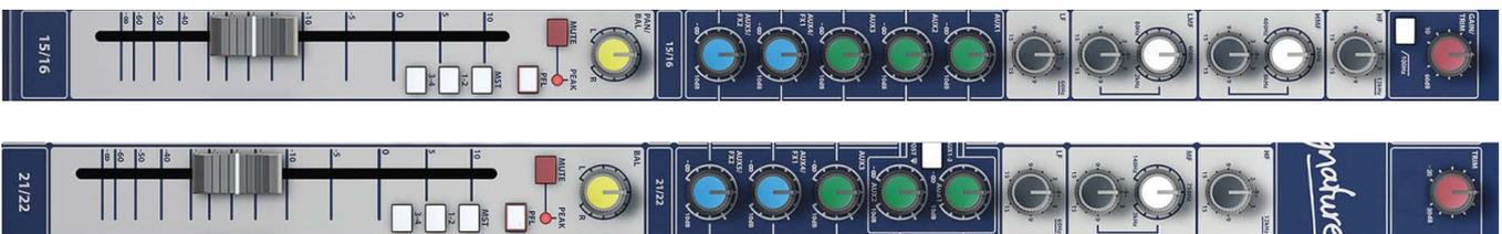
Signature 16, 22, and 22MTK consoles have two types of stereo inputs. One offers the option of a mono microphone/line level input by using either the XLR or Left/Mono Jack Input as well as stereo Jack inputs; the other (highest-numbered stereo channel) offers stereo line level phono inputs and is the 'Playback Channel'; the Master channel's INTERVAL MUTE function mutes all channels except the Stereo playback channel. Refer to Sections 4.3 and 5.3 for more detail.
