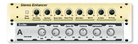
**ENHANCERS** let you emphasize the Bass, Midrange and Hi output at selectable frequencies, allowing you to generate maximum punch, clarity and detail – without turning up the overall volume. (Inspired by SPL Vitalizer\*)
