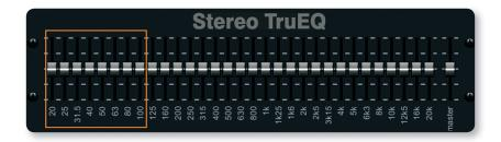
Unlike typical graphic EQs, our **STEREO TruEQ** delivers the exact frequency response for the new fader setting, taking neighboring fader settings into account – for surgical and responsive filtering or general room equalization (Modeled after BEHRINGER UltraCurve DEQ2496). The XR18 can provide up to 16 mono graphic EQs – one in each of the 6 Aux Buses and Main LR, plus 8 additional mono GEQ effects (4 stereo) that may be inserted into channels.
