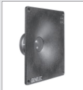
The tweeter driver is mounted in a DCW to match the dispersion characteristics to that of the bass driver. The DCW may be rotated for horizontal or vertical mounting.
