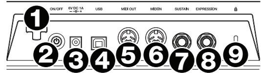
**Important:** If you use a USB charger to power Advance 49, set any relevant controls to send their MIDI messages out of the **MIDI Out**. Any controls set to transmit only over the **USB Port** will not be sent to a device connected to the **MIDI Out**.
