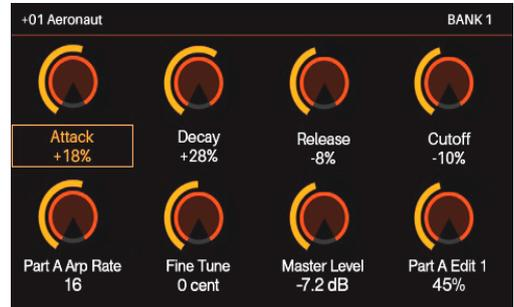
**MIDI Mode** shows you the current settings of Advance 49's controls when used with your DAW (or an external MIDI device). Press **Shift** and the **Control (MIDI)** mode button to enter it.
