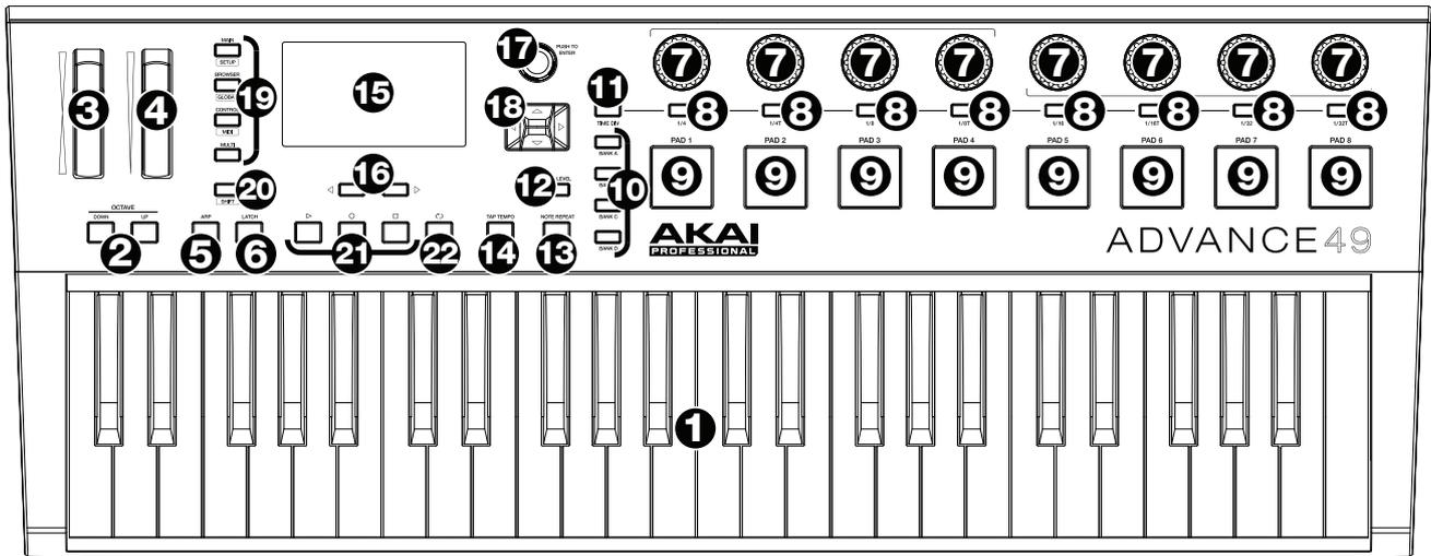
1. **Keyboard:** This 49-note keyboard is velocity- and pressure-sensitive and, in conjunction with the **Octave Up/Down** buttons, can control a 10-octave range.
