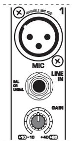
Fig. 2.1: Connectors and controls of mic/line inputs
