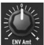
The **ENV Amt** lets you control the amplitude and polarity of the envelope signal sent to modulate the filter cutoff frequency. At the 0 position (12 o'clock), no envelope modulation occurs. When turned counter-clockwise (below the 0 mark), the **ENV Amt** knob sends an increasing amount of the inverted ADSR envelope. When turned clockwise (beyond the 0 mark) the **ENV Amt** knob sends an increasing amount of the standard, positive-going ADSR envelope.
