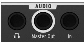
Connect the **Master Out** with an unbalanced audio cable to an audio mixer, a computer's sound card, or directly to an audio amplifier. The **Master Volume** knob [4.2.8.6] controls the output level.
