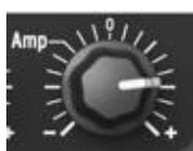
The **Amp** knob control the amplitude and polarity of the LFO signal that modulates Amplifier's level. On the 0 position (12 o'clock) no modulation is sent to the target. When turned counter-clockwise (below the 0 mark) the **Amp** knob sends an increasing amount of the inverted LFO signal. When turned clockwise (beyond the 0 mark) the **Amp** knob sends an increasing amount of the normal LFO signal.
