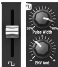
The level of the plain Square wave and Pulse width modulated signals is controlled with the slider potentiometer labeled with the square symbol. Pulling it down completely mutes the signals and moving it up increases their level. When the **ENV Amt** (envelope amount) knob is set to 12 o'clock (0 mark) and the **Pulse Width** knob is fully counter-clockwise (50% tick), the square wave is audible.
