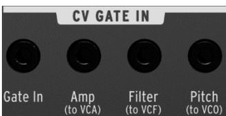
The MiniBrute also connects with other analog devices (analog synthesizer, analog step sequencer, etc.) through a **CV/GATE** interface where **CV** means Control Voltage. The **Gate In** 1/8" jack allows other analog devices to trigger the MiniBrute envelopes. The main MiniBrute functions (i.e., amplifier volume, filter cutoff, and oscillator pitch) are controlled by the **Amp (to VCA)**, **Filter (to VCF)** and **Pitch (to VCO)** 1/8" jacks respectively.
