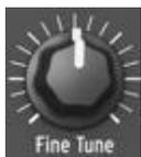
The **Fine Tune** knob provides precision adjustment of the oscillator pitch. The 12 o'clock position corresponds to the default tuning (i.e. A=440Hz) when you play the second rightmost A of the keyboard and the default **Octave** [4.2.8.3] is selected. The full range of the **Fine Tuning** knob is from about -2 semitones to +2 semitones. Fine-tuning makes it possible to tune the MiniBrute to other instruments that are slightly out of tune.
