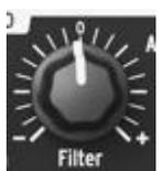
The **Filter** knob controls the amplitude and polarity of the LFO signal that modulates the filter's cutoff frequency. At the 0 position (12 o'clock) no modulation is sent to the target. When turned counter-clockwise (below the 0 mark) the **Filter** knob sends an increasing amount of the inverted LFO signal. When turned clockwise (beyond the 0 mark) the **Filter** knob sends an increasing amount of the normal LFO signal.
