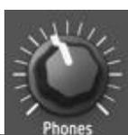
The **Phones** knob controls the volume of the Phones output located on the rear panel [4.3.3]. Remember to be cautious with levels when
