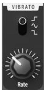
The Vibrato is a specialized low frequency oscillator dedicated to oscillator pitch modulation. It's completely independent from other modulation sources, and its modulation depth and triggering are controlled by the **Modulation** wheel [4.2.4.1] and the **Aftertouch** switch [4.2.4.2] respectively. It provides different modulation waveforms, selectable with a three-position switch:
