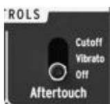
The **Aftertouch** switch controls the aftertouch signal assignment; aftertouch is very useful to trigger modulation events while playing without using extra knobs or sliders, thus increasing expressiveness. The **Aftertouch** switch has three positions: it can be routed the filter cutoff frequency (**Cutoff**), used to trigger **Vibrato** [4.2.5], or be disabled (**Off**).
