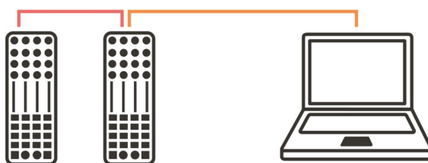
K1 CONTROLLERS via X:LINK + LAPTOP via USB
