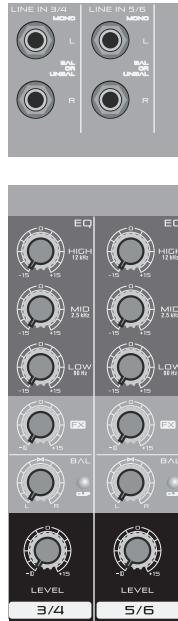
Fig. 2.2: Connectors and controls on the stereo channels
