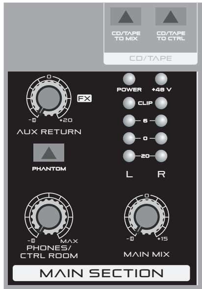
Fig. 2.4: Control elements of the main section
