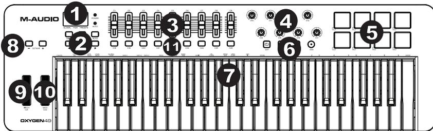
1. **LED Screen:** The Oxygen 49 features a 3-digit LED display providing visual information regarding current operation, programming and controller status.
