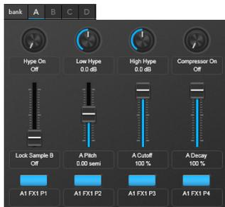
The Assignable Controls in Arsenal reflect the current parameters and settings or positions of Trigger Finger Pro's **Assignable Knobs**, **Assignable Faders**, and **Assignable Buttons** across all four banks (A–D).
