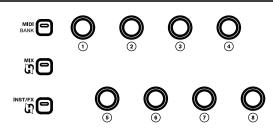
**HyperControl Mix Mode:** Press the **Mix** 🖏 button next to the knobs to switch them between three functions in HyperControl Mix Mode:
