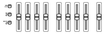
**Important:** Only Axiom AIR 49 and Axiom AIR 61 have the eight faders described in this section. All three keyboards, however, have a master fader. In *both* modes, the master fader will control your Cubase session's master volume level.
