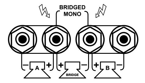
As shown in the graphic above, the stereo and bridged mono applications can be connected as indicated. Binding post wiring can be done with spade connectors, bare wire ends tightened into the binding posts or via banana plugs inserted into the end of the binding posts.
