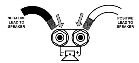
Strip away approximately ½" (12mm) of insulation from the speaker wire. Twist the bare copper wire ends tightly. Unscrew each binding post, insert the wire into the hole in the metal portion of the binding post and tighten the binding post securely. Be care of stray wire strands that could cause shorts.
