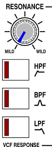
**18 Adjust the filter resonance.** Slowly turn the RESONANCE control clockwise as you sweep the frequency and you should hear the 'Q' or 'sharpness' of the effect changing from subtle to drastic as the roll-off knee sharpens and frequency boost is added.
