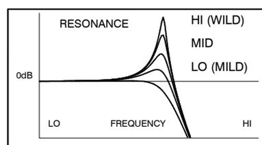
**High RESONANCE settings can result in significant boost of selected frequencies. Reduce the channel GAIN if the signal levels increase enough to light the red PK leds in the output meters. Failure to do this may result in system overload and distortion.**
