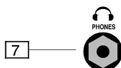
**4 HEADPHONES level control.** Adjusts the level of the signal in the stereo headphones. This does not affect the level of the local monitor.
