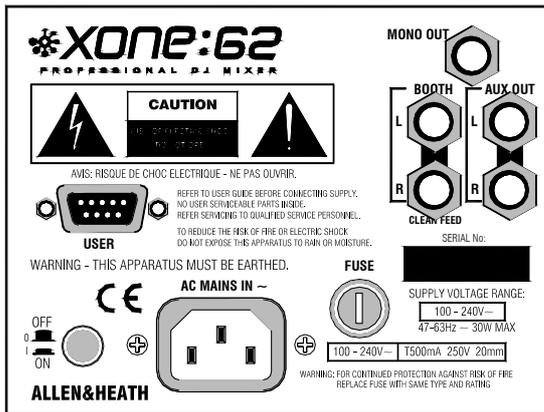
Read the **SAFETY INSTRUCTIONS** printed at the front of this User Guide and on the rear panel. Check that the correct mains lead with moulded plug has been supplied with your console. The power supply accepts mains voltages within the range 100-240V without changing any fuses or settings.
