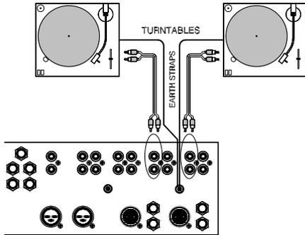
**15 Crossfader mixing.** At this point you may wish to plug in a pair of turntables and experiment with DJ mixing. Plug into CH3 and CH4 phono inputs if your turntables require RIAA equalisation. If not, plug into the line inputs. Remember to connect the turntable earth leads to the console chassis earth terminal. Use CUE to set up the channel gain as you did in step 7. Route CH3 to X and CH4 to Y of the crossfader.
