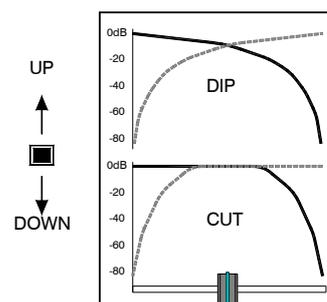
**4 XFADE ON.** In the up position the music signal is routed directly to the mix. Press to route the signal through the crossfader.
