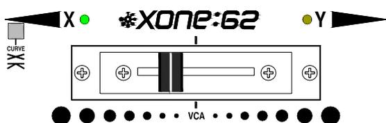
**13 Using the Crossfader.** This lets you fade between signals routed to either side, typically to fade smoothly into a new music track or to creatively layer sounds when scratch or cut mixing. Experiment further by connecting two CD decks or turntables and assigning one to X, the other to Y. Use XFADE PAN to adjust the balance between the left and right mix, either to correct an imbalance or as an effect in its own right.
