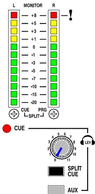
**8 Check the sound using the Cue system.** With the music playing press the large CUE switch. The switch lights as well as the master CUE led to show that the cue monitor is active. The channel signal is now sent to the headphones. Slowly turn up the headphones level control until you hear the music.
