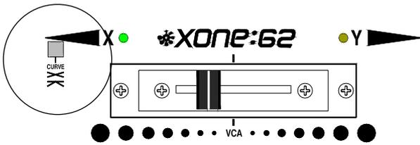
**14 Changing the crossfader curve.** The little switch to the left of the crossfader sets which curve is active. In the normal up position the signal dips by 6dB at the middle position for smooth fading between tracks. Press the switch for a dipless response where the signal starts to dip only once the fader has passed the mid position. This is better suited to scratch or cut mixing where you layer the sounds.
