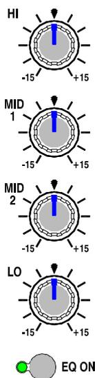
**11 Check the effect of the Stereo EQ.** Press CH3 EQ ON switch. This lights to show that the signal is routed through the equaliser. Now try the effect of each of the 4 frequency bands. The EQ is designed for creative live performance control and provides a safe +6dB boost and a massive -26dB cut. Experiment with cutting rather than boosting frequencies to create dramatic effects. These can be punched in or out using the EQ ON switch.
