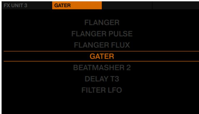
5. Turn the **BROWSE** encoder to select any FX and press the **BROWSE** encoder to assign the FX.
